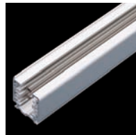
Three-phase surface track L1+L2+LB+N+TT 16A/400V
